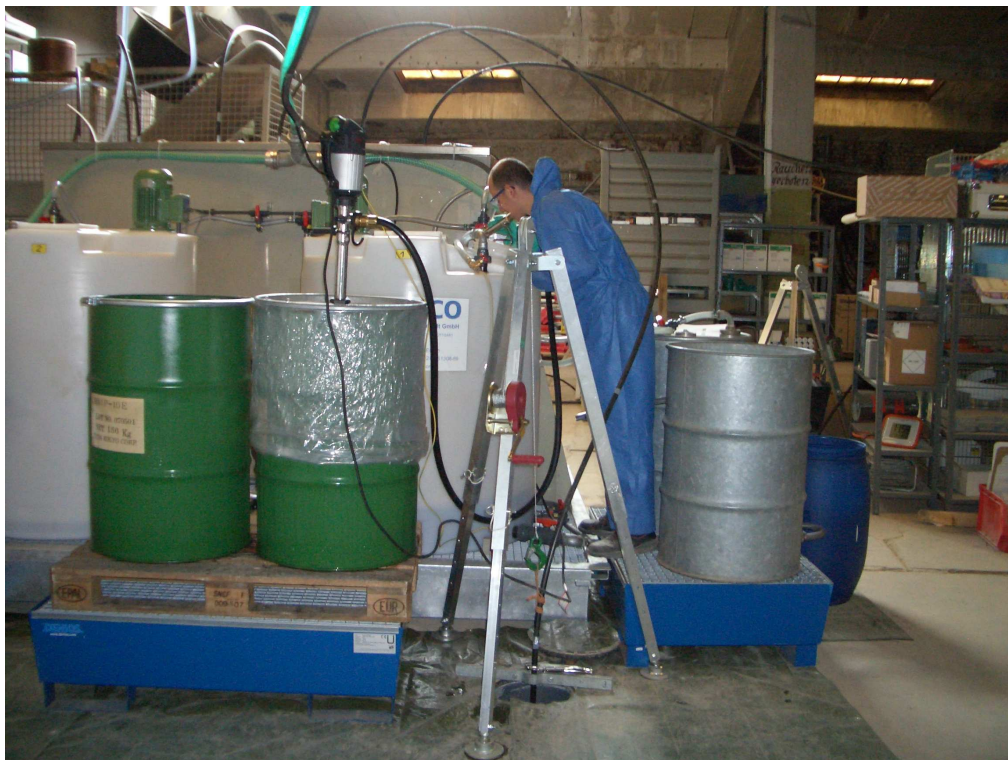
Fig. 9: Set up at the site (indoor). Stirring tanks for nZVI resuspension. © Alenco GmbH, Germany
