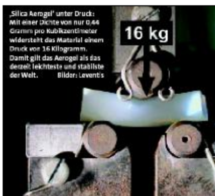
Fig. 4: Aerogel material with improved mechanical properties 27 (Automobil Entwicklung)
